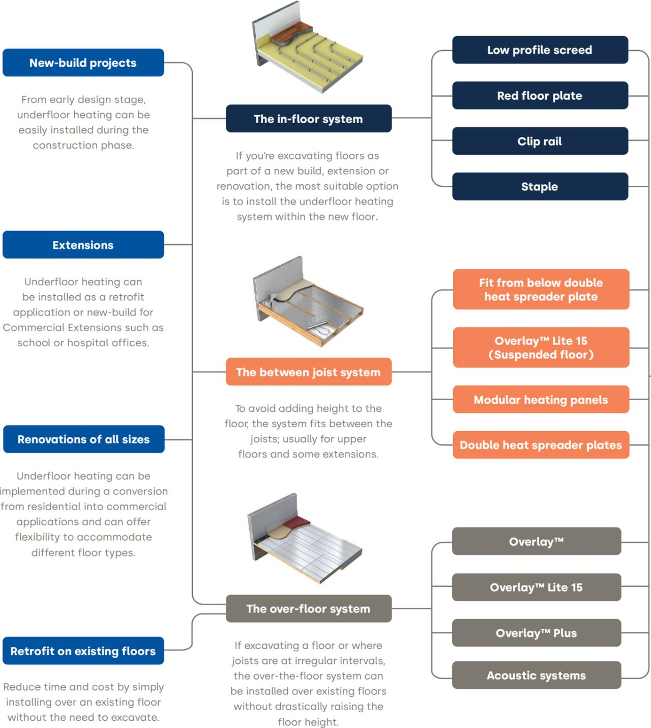
Introducing our system portfolio. From our traditional Staple and Clip Rail systems to our over-the-floor and between-the-joists systems, you have the flexibility for any underfloor heating application.
